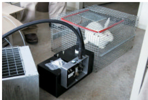
Figure 2. Tunnel-like link to nesting box, including a door to be operated by a chip
