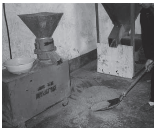
Figure 4. Small pelleting machine at work in China, with an electric engine (protected inside the box below the pelleting device), loaded by hand
