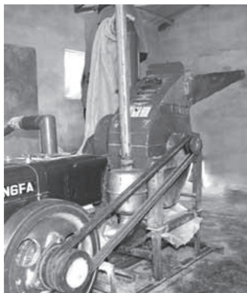
Figure 3. Small forage grinding machine at work in Benin, with a diesel engine, loaded by hand
